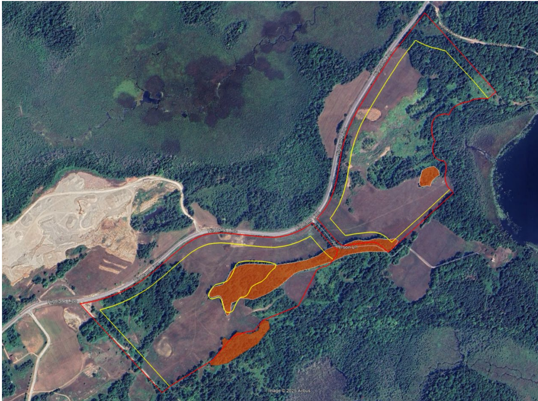
Figure 1: Interpreted Area of Exposed and/or Shallow Bedrock Observed August 2025. (Orange polygons represent areas of exposed and/or shallow bedrock)
